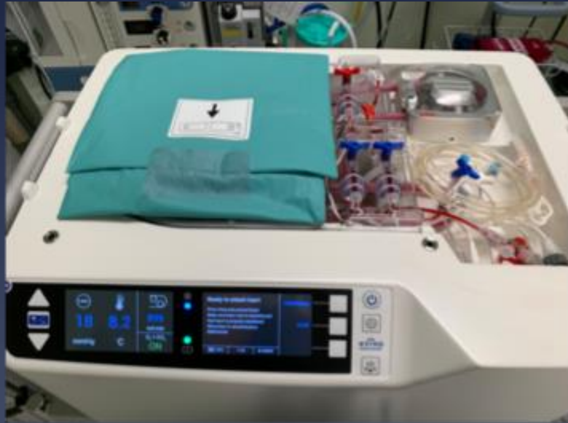
Image 1. The HOP machine primed with blood-based perfusate (left) and attached to a heart (right). (Photos taken during the first HOP preservation run.)
